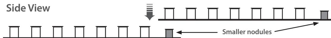
Each panel has one long and one short edged with smaller nodules (marked by darker circles between each nodule).
