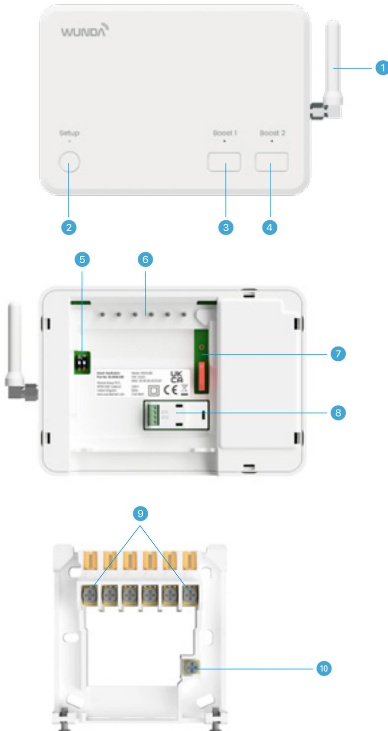
1- **Antenna**; 2 - **Setup** button; 3 - configurable **Boost 1** button; 4 - configurable **Boost 2** button; 5 - **Switch**; 6 - Backplate connectors; 7 - **Jumper**; 8 - **OpenTherm** connector; 9 - Backplate wire connectors; 10 - Ground
