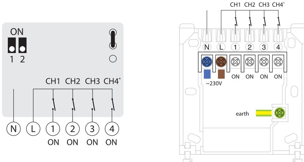
\* CH4 can be configured for either heating or hot water in the application
